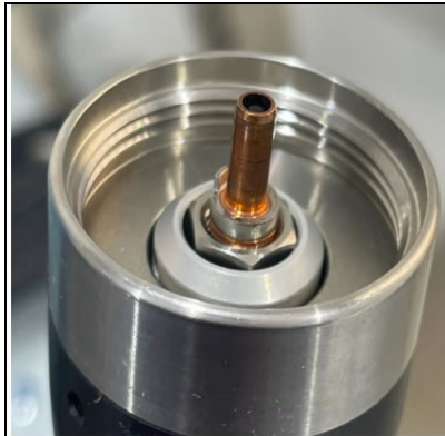
Correct fiber position: The end of the fiber is located in the crater of the ferrule.
