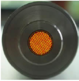
Coherent and randomized silica fiber bundle
