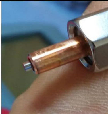
Incorrect fiber position: Fiber protruded of the ferrule
