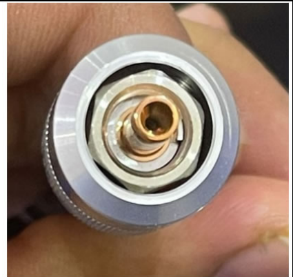
Incorrect fiber position: Fiber pulled inside the ferrule
