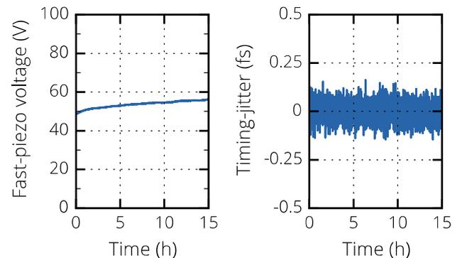
Figure 3 — Passive stability of both lasers: Evolution of the fast-piezo compensation voltage (left) and recorded in-loop timing-jitter (right) along 15 hours. RMS timing-jitter is 41 as.
