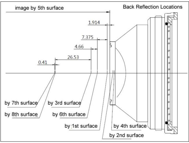
For laser marking applications, M1 and M2 may not be exactly same as the designed parameters. The allowed tolerance may be around 6-10mm, which does not result in obvious changes of marking performance.
