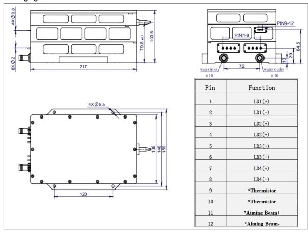
1. STK Serie s blue laser consi sts of up to 4 subm odule s 50 W per modul e ) . Powe r can be suppli ed separ ately m
