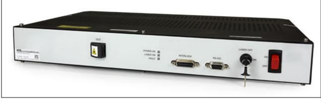
A series of high-power spectrally-sliced Erbium Broadband Sources providing up to 100 channels (50 GHz) locked to the ITU grid at 22 dBm output power. This source can dramatically reduce equipment cost and setup time in DWDM system test, replacing costly banks of DFB lasers.
