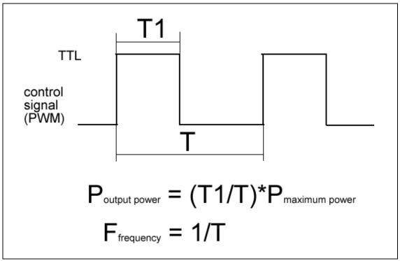
In our controllers, the frequency is fixed at 5kHz (0.2ms). Adjusting the output laser power means adjusting pulse width T1.
