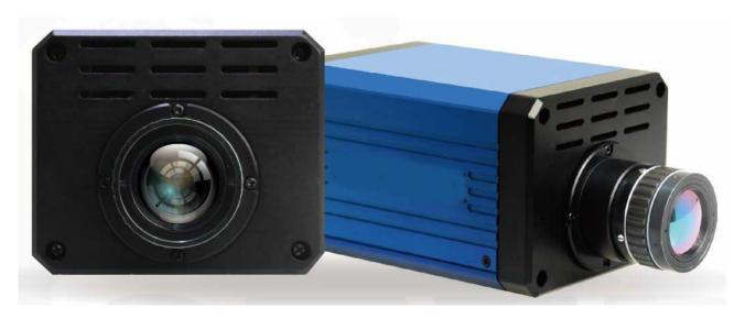
STL series MWIR camera is developed with resolution 640x512pixels, wavelength range 3.7~4.8um, standard CL connector, supporting standard analog PAL video and external trigger. The camera is Stirling refrigerator cooled and provides with 14bit and 117Hz output.
