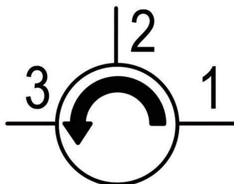
Circulators can be used to achieve bi-directional transmission over a single fiber. Because of its high isolation of the input and reflected optical powers and its low insertion loss, optical circulators are widely used in advanced communication systems and fiber-optic sensor applications.
