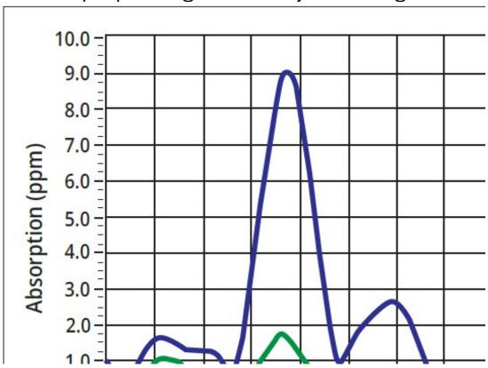
Graph clearly highlights that surface absorption at 532nm performed on coated LBO Superpolished crystal (roughness <3Å) is about 4 times less absorbent than standard polished coated LBO crystal (roughness of ~10Å). Based on this difference, LBO Superpolished crystals made by us should exhibit longer lifetime.
