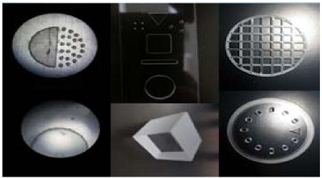
Sub-surface engraving and cutting of fragile glasses
