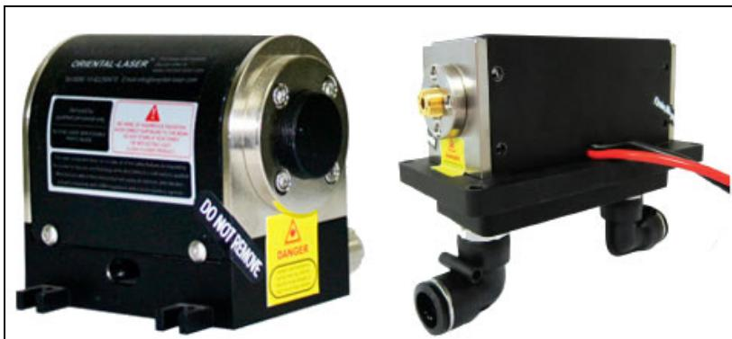
The work mode of gain modules is CW or QCW. The QCW module also includes conduction cooling module and water cooling module. STO series CW module maximum power is 450W. Much powerful module also can be customized upon request. Typical applications are laser amplifiers for nanosecond and picosecond MOPA lasers, gain modules for unstable oscillator resonators, CW pumped, 532nm, ns q-switched lasers, and LIDAR lasers.
