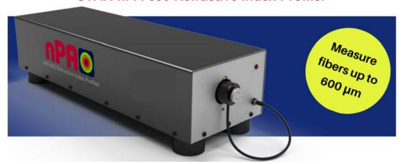
Our refractive index profiler uses a modified refracted near-field technique to analyse a fiber end-face to determine the full 2D refractive index distribution. The STAR-nPA-600 is the quick and easy way to get the refractive index data you need to verify your specialty fiber design and manufacturing processes. The instrument comes with the v2.0 software which boosts system performance and improves user experience, and the API allows the STAR-nPA-600 to integrate to other system seamlessly.
