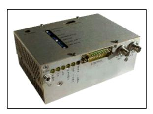
where the mode of operation is defined by ZZZ = A05 normal analog mode, or R05 analog switched to full RF mode or a triggered RF ramp down mode where ZZZ = FPS first pulse suppression mode or PPK pre-pulse kill mode. The choices of frequency (XX), output power (YY), and power control (ZZZ) option are "factory set" when ordered. The driver requires forced air cooling.
