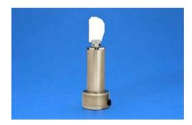
The 6230H galvanometer can be designed and optimized for speed, size, cost and accuracy with typical beam diameters of 8mm, 10mm, 12mm, and 15mm. It is shown here with a 10mm Y mirror.
