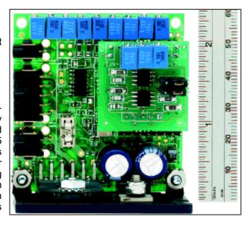
Designed with flexibility in mind, the MicroMax Model 677XX features differential analogue inputs, flexible power supply configurations and positioning control allowing for optimization of system positioning angles, speed and accuracy. System position, velocity and error output signals make integrations into complex scanning system applications easy and accurate. Integral mounting hardware, low profile connectors and the overall small size allow for compact system designs with easy integration.
