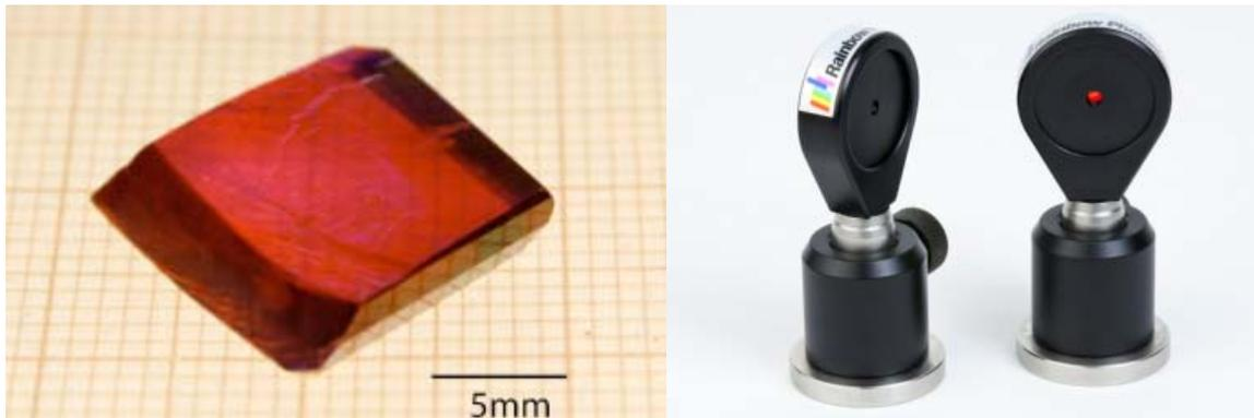
Example of an as-grown **STRP-OH1** crystal and organic crystals polished, coated and mounted for optical applications. **STRP-OH1** and other high-quality organic crystals are produced and optically prepared in the facilities of Rainbow Photonics in Switzerland.
