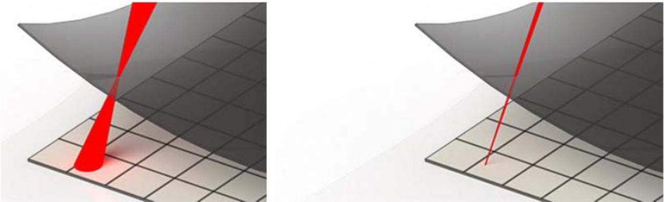
Figure 5: The left panel shows the defocused laser spot on the marking plane. By tuning the EL-10-42-OF the laser spot remains focused on the marking plane, see right panel.
