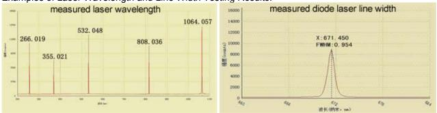
Examples of Laser Excitation Spectrum Testing Results:
