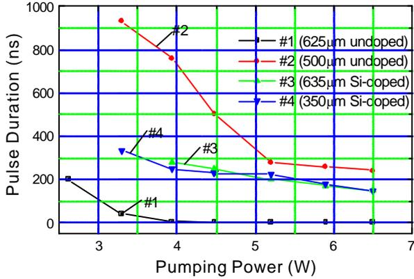
Fig. 5 Variation of pulse duration with the increase in pumping power for different wafers.
