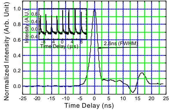
Fig. 6 A pulse of 2.6 ns in pulse duration and a pulse train of 300 kHz in pulse repetition rate produced by the passive Q-switching using wafer #1.
