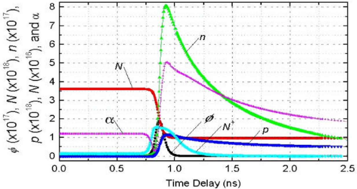
Fig. 7 simulated results using the combined F-P and energy-level models
