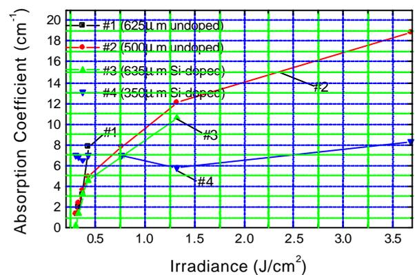
Fig. 2 the measured absorption coefficient of GaAs wafers with the increase in the intensity of the incident laser beam
