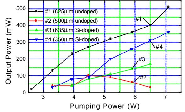
Fig.4 Averaged output power for different GaAs wafers
