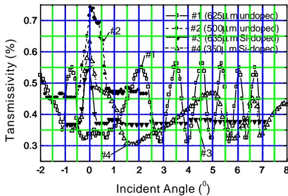
Fig.1 The measured transmissivity of GaAs wafers with the variation in incident angle
